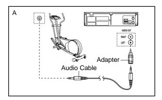
B. Plug one end of the audio cable into the jack beneath the console of the elliptical crosstrainer. Plug the other end of the cable into the included adapter. Plug the adapter into an RCA adapter (available at electronics stores). Next, remove the wire that is currently plugged into the AUDIO OUT jack on your VCR and plug the wire into the unused side of the RCA adapter. Plug the RCA adapter into the AUDIO OUT jack on your VCR.
